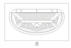
it is recommended to install vertically against the wall 2-3m high above the ground as picture ①shown
